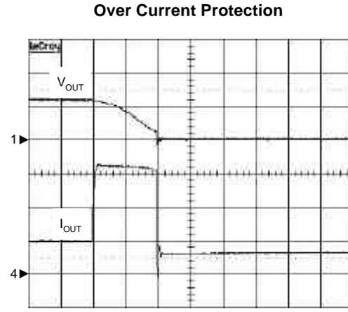
$C_{OUT}=10\mu F$ ,  $C_{IN}=10\mu F$ ,  $I_{OUT}=1A$  to  $3.4A$
