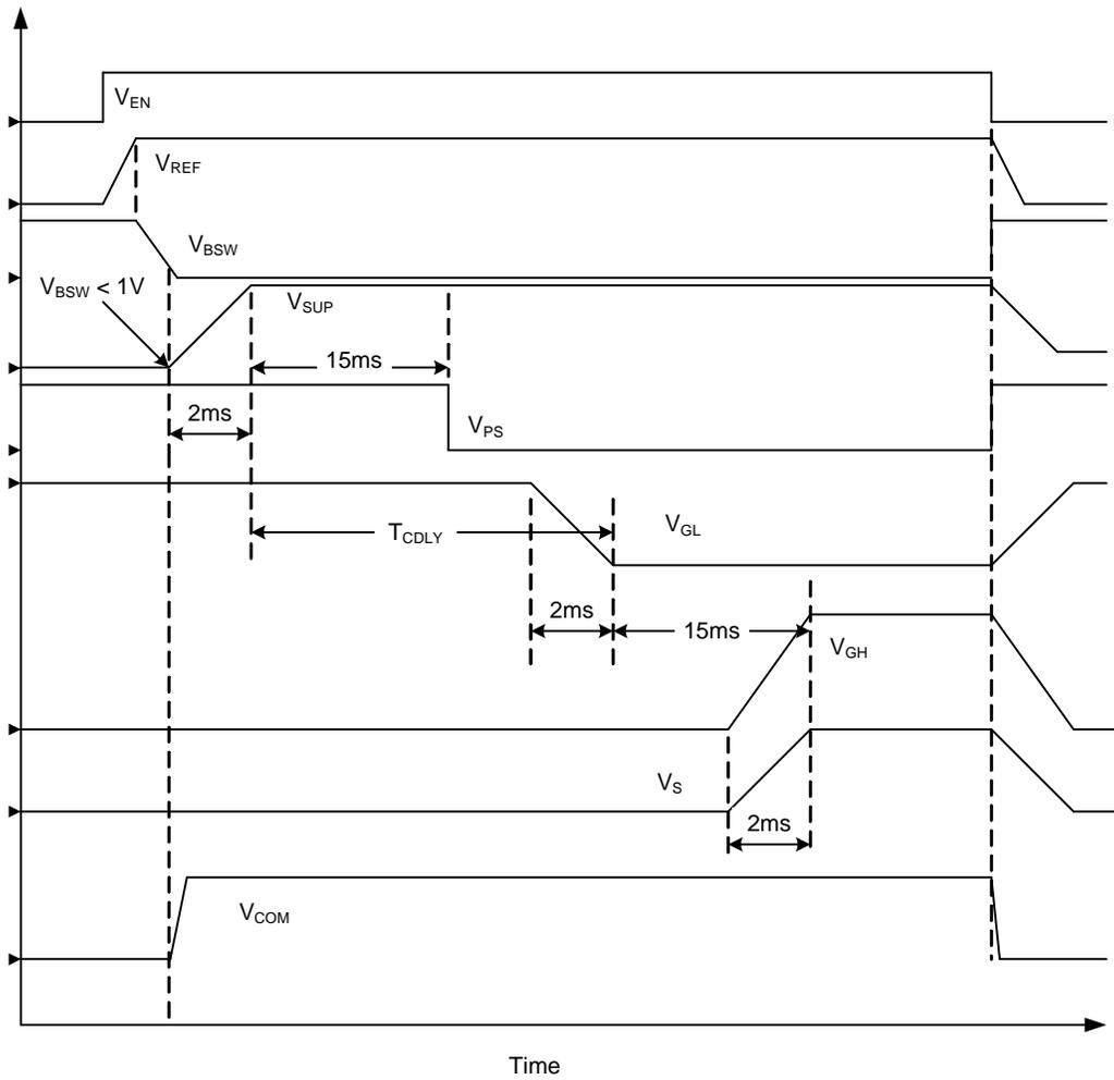
The output voltage falling slew rate after shutdown depend on external resistance beside  $V_{COM}$ .
