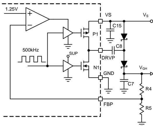
Fig1. Positive Charge Pump Regulator Block Diagram
