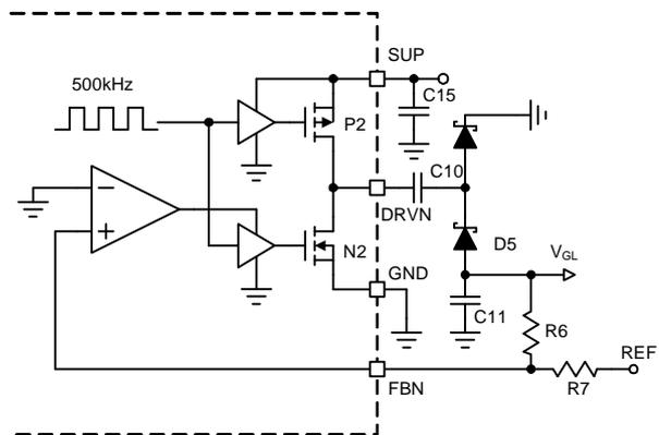
Fig2. Negative Charge Pump Regulator Block Diagram
