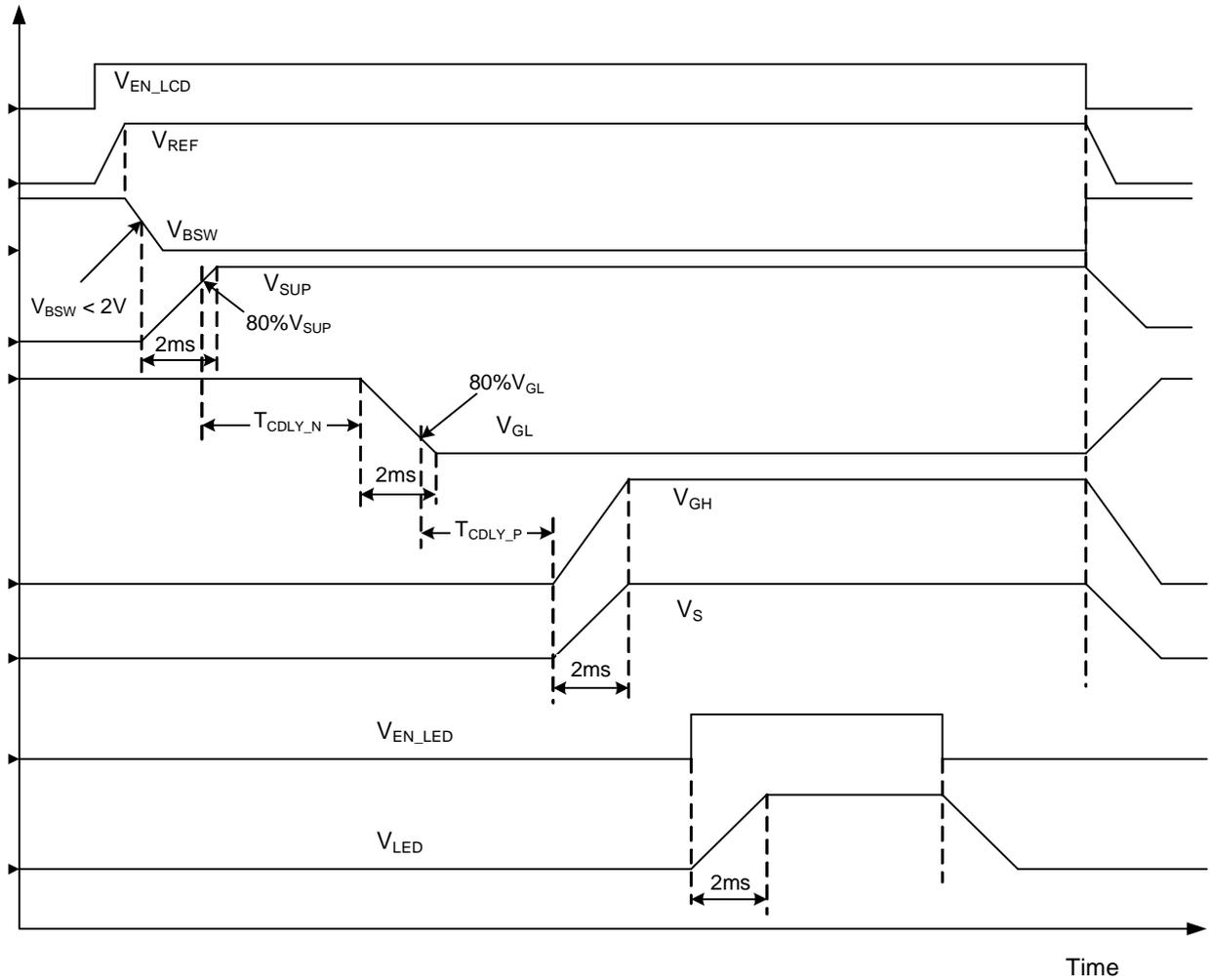
The output voltage falling slew rate after shutdown depend on external resistance.
